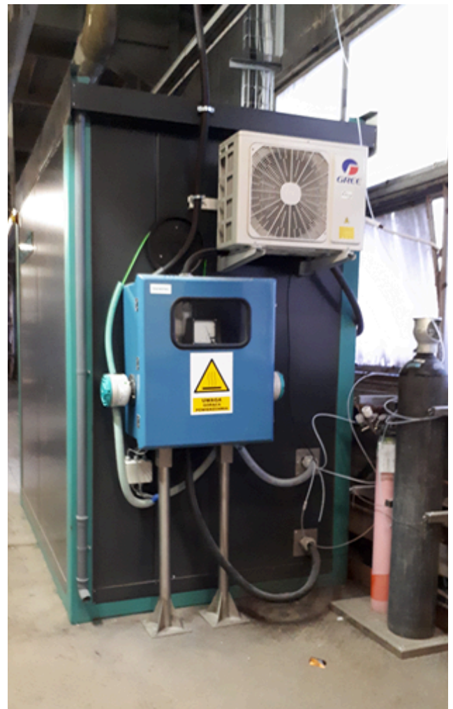
Fig. 14. Conditioned cabinet with a built-in laser spectroscopy - NH 3 analysis
