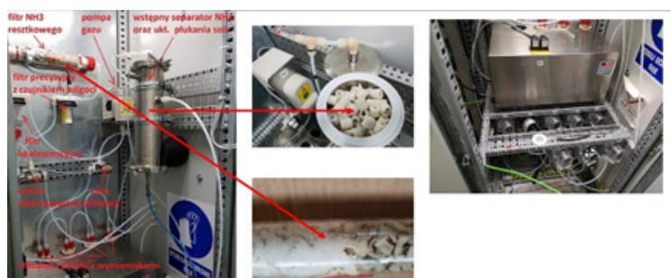
Fig. 7-10. Elements of the "cold" CO 2 analysis system
